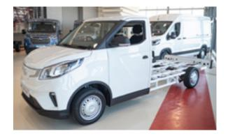
CHASSIS (5156mm Max Overall Length (1810mm Max Body Width)
